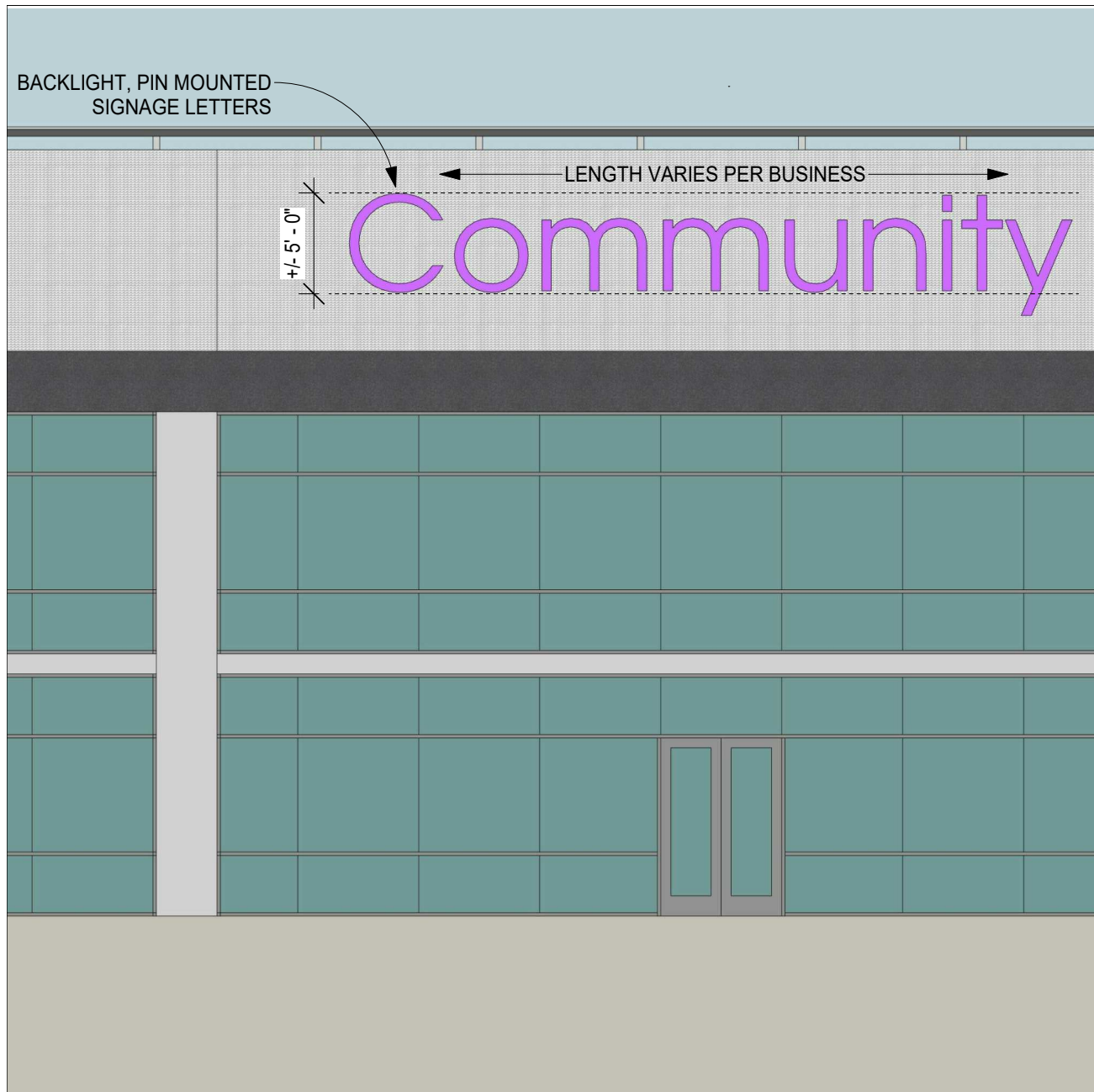
3 Wall Sign Elevation 1/8" = 1'-0"
