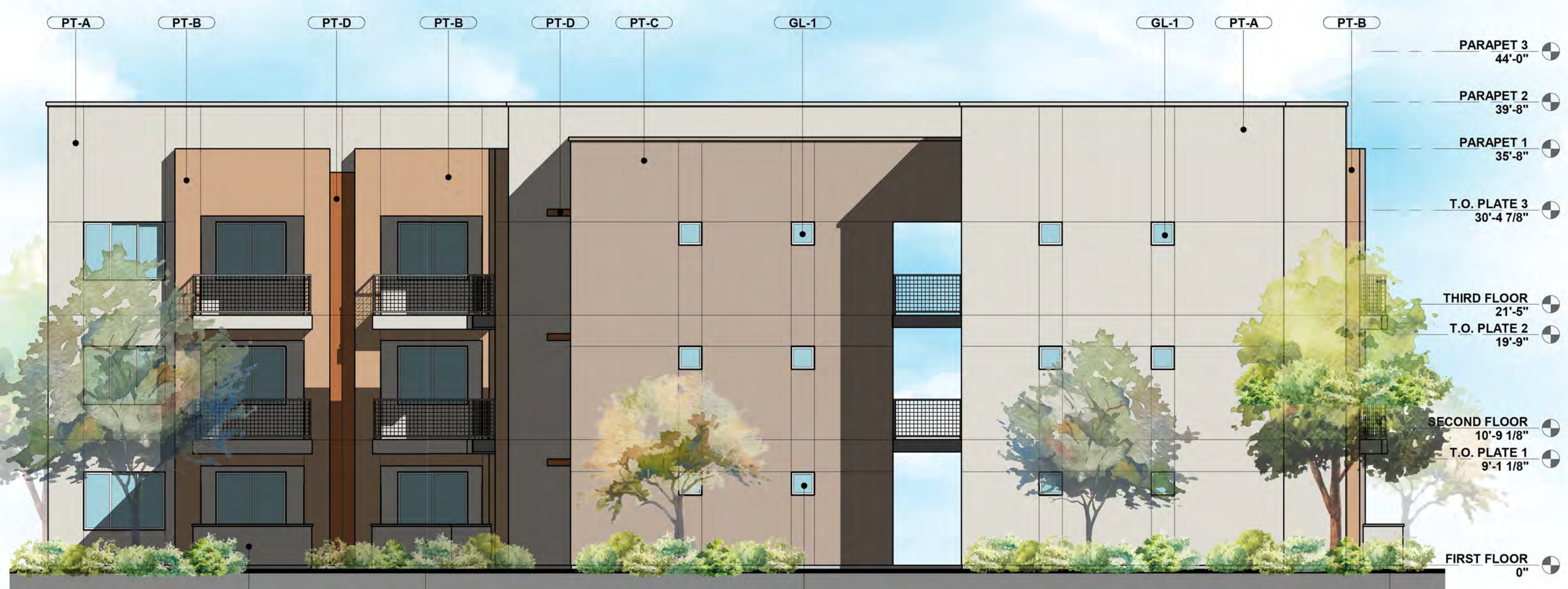
2 BUILDING 4 LEFT ELEVATION 1/8" = 1'-0"
