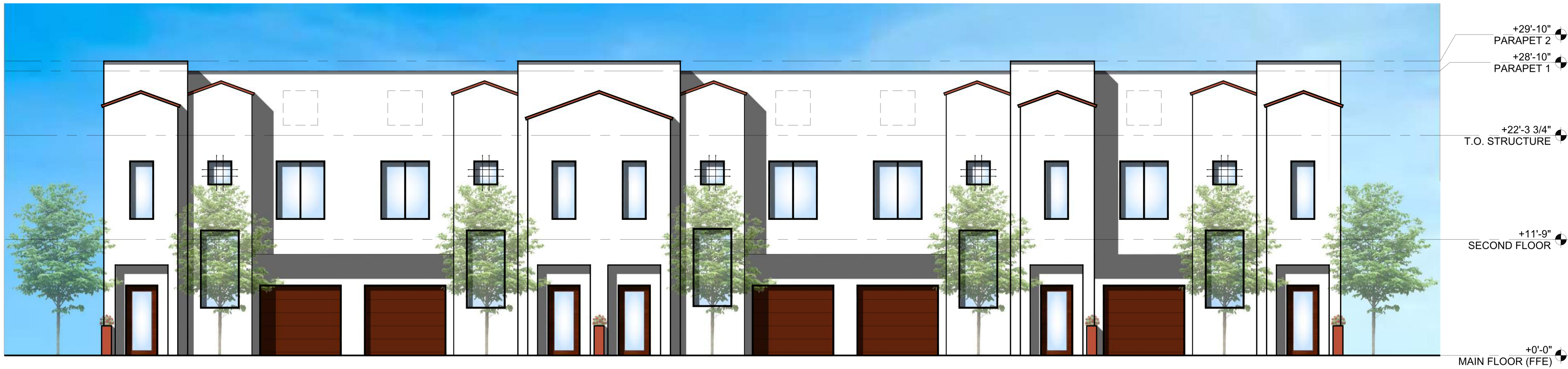
1 BLDG 5 - FRONT ELEVATION 1/8" = 1'-0"
