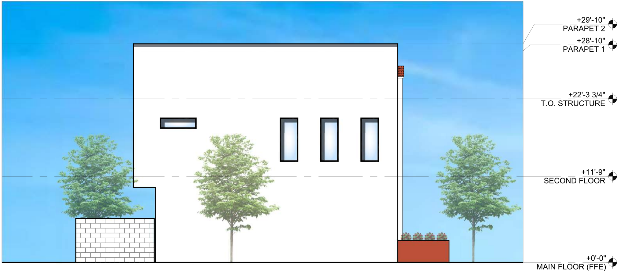
4 BLDG 6 - SIDE ELEVATION 1/8" = 1'-0"
