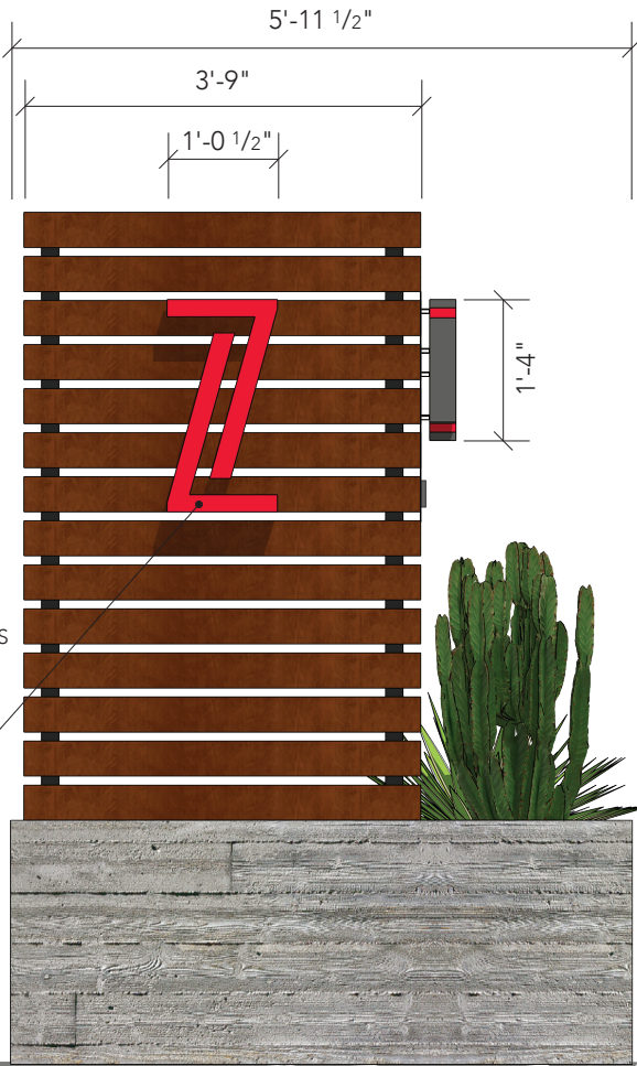
REVERSE-LIT CHANNEL LETTER SECTION NTS
