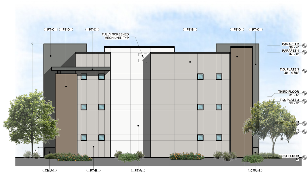
2 BUILDING 1 SIDE ELEVATION 1/8" = 1'-0"
