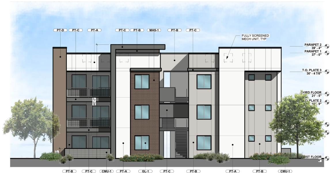
1 BUILDING 3 FRONT AND REAR ELEVATION 1/8" = 1'-0"
