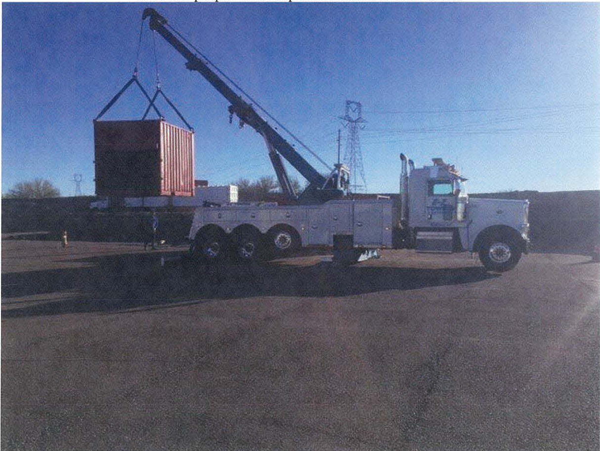
Using our 50 Ton Rotating Wrecker, we were able to assist the local Fire Department with the assembly of the new "Flash Over" chamber at the Avondale/Goodyear Fire Training Facility.
