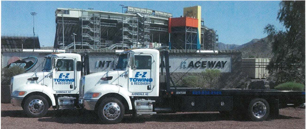
Flatbed "Rollback" Style Tow Trucks at ISM Raceway Avondale, AZ.
