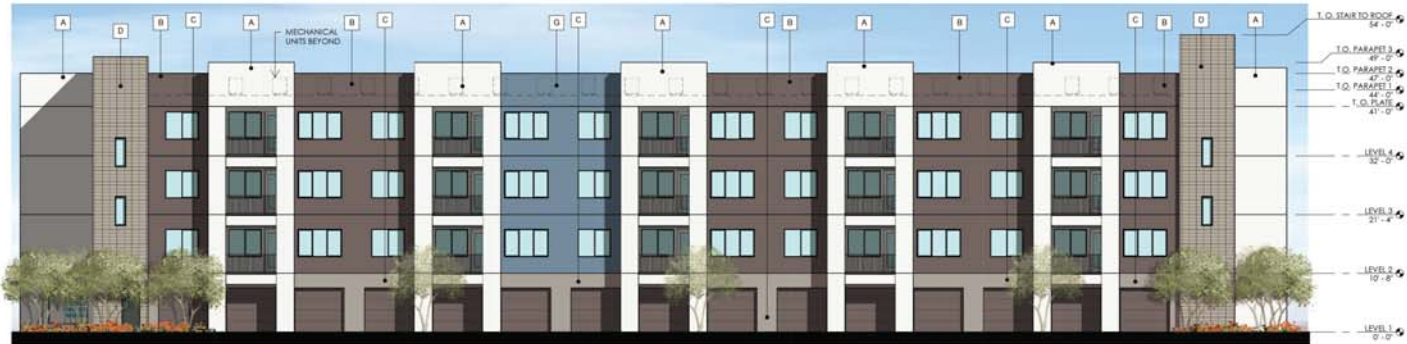
2 BUILDING 4 - NORTH ELEVATION 3/32" = 1'-0"
