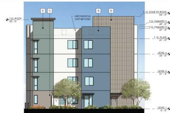
3 BUILDING 3 - EAST ELEVATION 3/32" = 1'-0"
