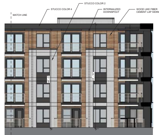
BUILDING A - COURTYARD SOUTH ELEVATION 1/8" = 1'-0"
