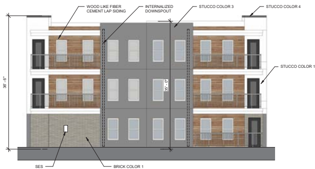
2 A-008 BUILDING C1 - SOUTH ELEVATION 1/8" = 1'-0"
