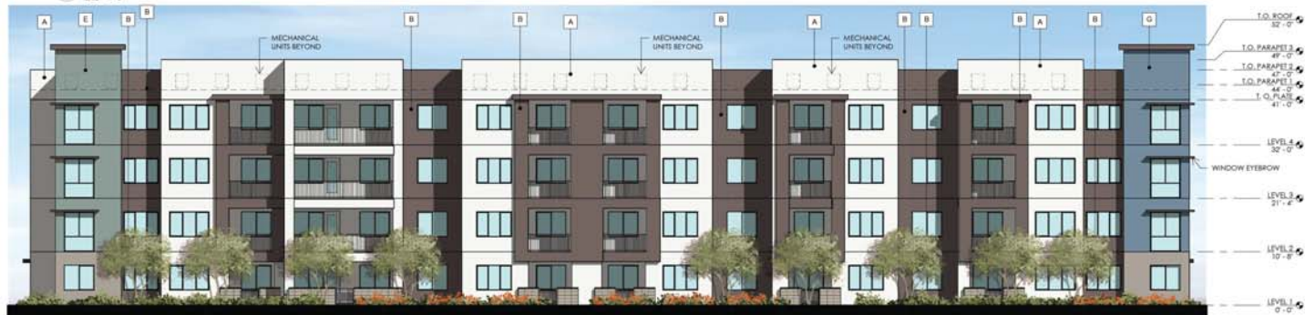
1 BUILDING 4 - SOUTH ELEVATION 3/32" = 1'-0"
