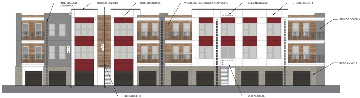
BUILDING B1 - EAST ELEVATION A-007 1/8" = 1'-0"
