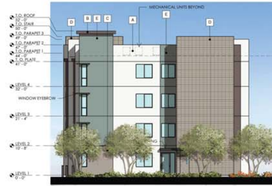
4 BUILDING 1 - SOUTHEAST ELEVATION 3/32" = 1'-0"
