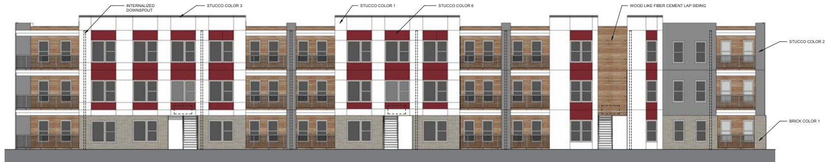
4 A-008 BUILDING C1 - WEST ELEVATION 1/8" = 1'-0"
