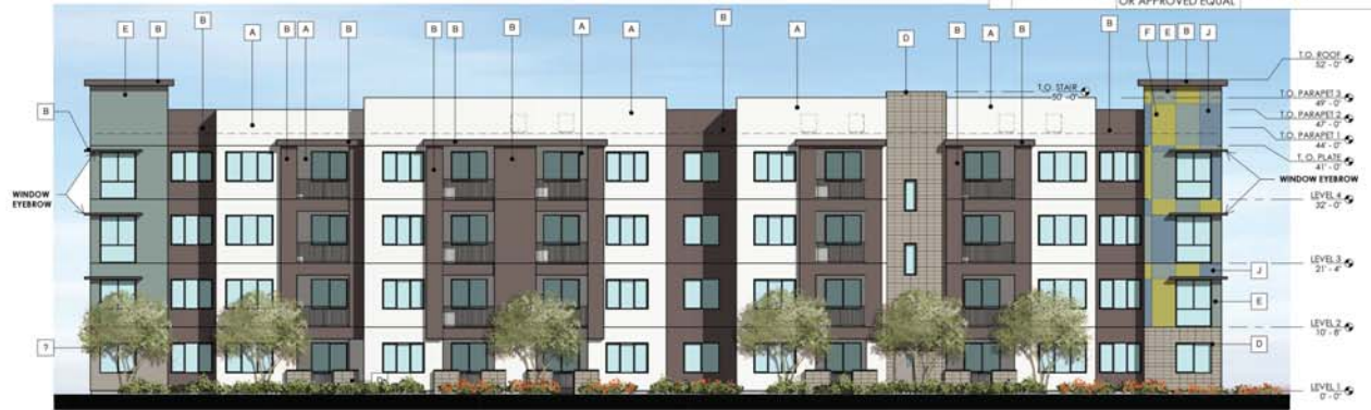
1 BUILDING 6 - NORTH ELEVATION 3/32" = 1'-0"
