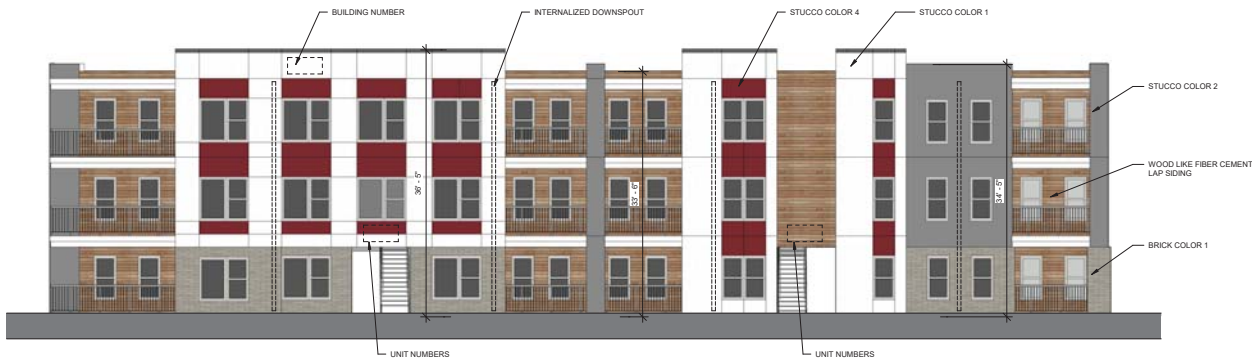
BUILDING B1 - WEST ELEVATION A-007 1/8" = 1'-0"
