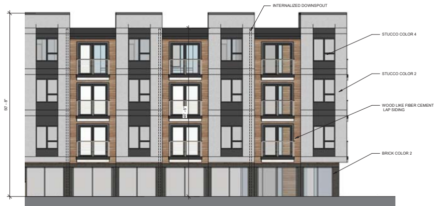
3 A-001 BUILDING A1 - COURTYARD EAST ELEVATION 1/8" = 1'-0"
