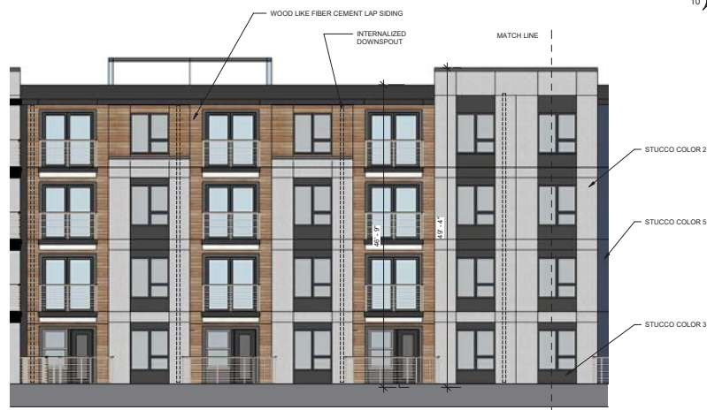
6 A-003 BUILDING A1 - COURTYARD NORTH ELEVATION 1/8" = 1'-0"
