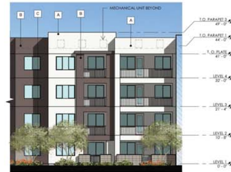
1 BUILDING 1 - EAST ELEVATION COURTYARD 3/32" = 1'-0"
