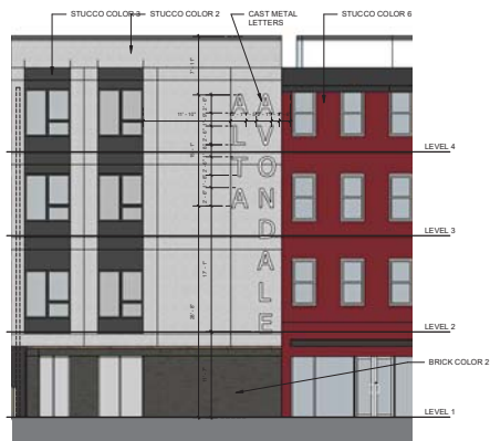
3 BUILDING A1 - SOUTH ELEVATION WALL SIGN A-014 1/8" = 1'-0"
