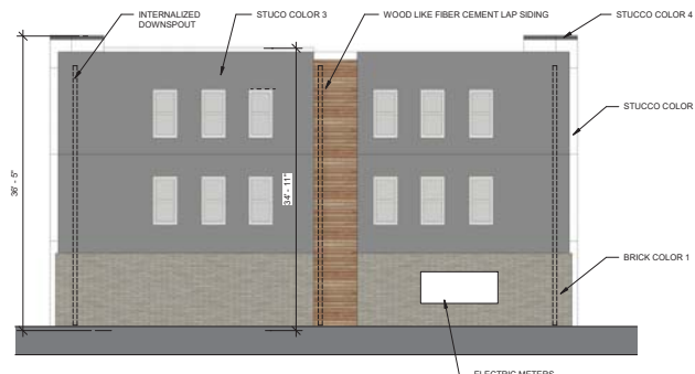
3 A-008 BUILDING C1 - NORTH ELEVATION 1/8" = 1'-0"
