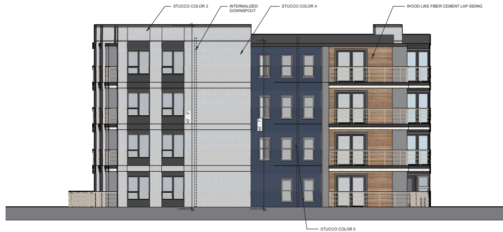
13 A-006 BUILDING A1 - EAST ELEVATION 1/8" = 1'-0"
