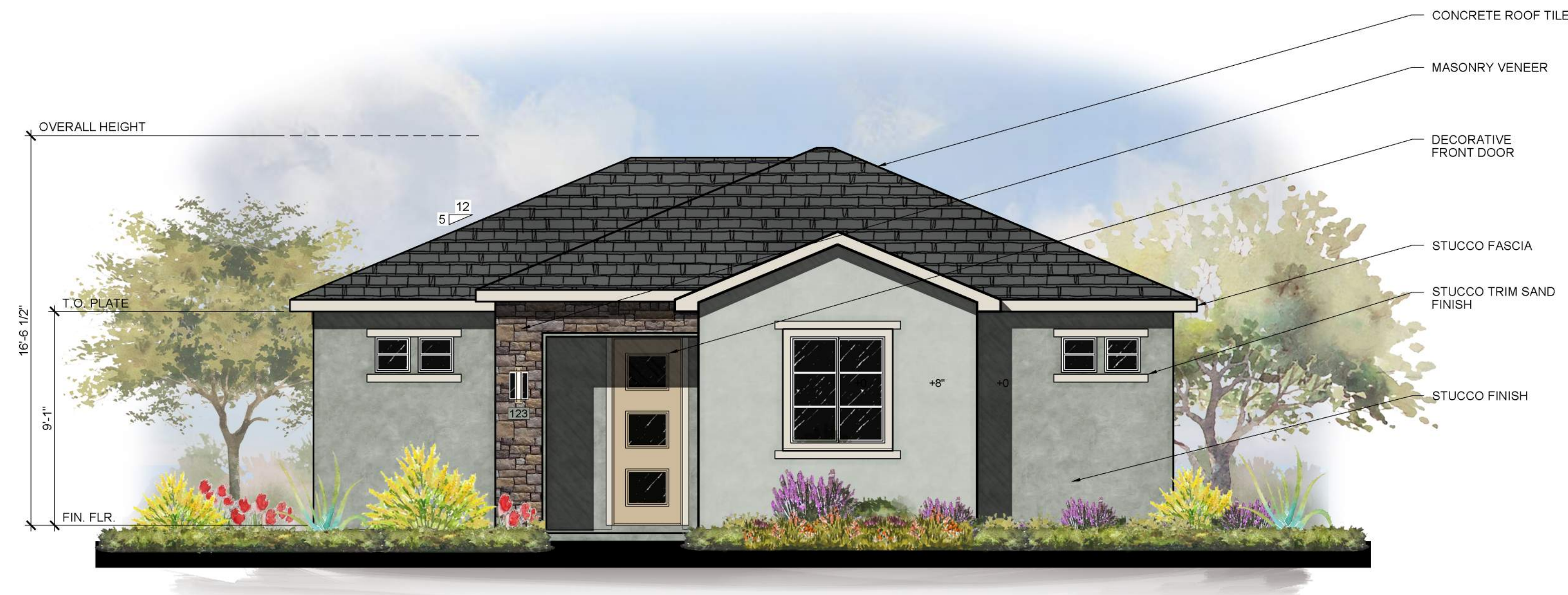
Front Elevation Elevation C 1/4" = 1'-0"
