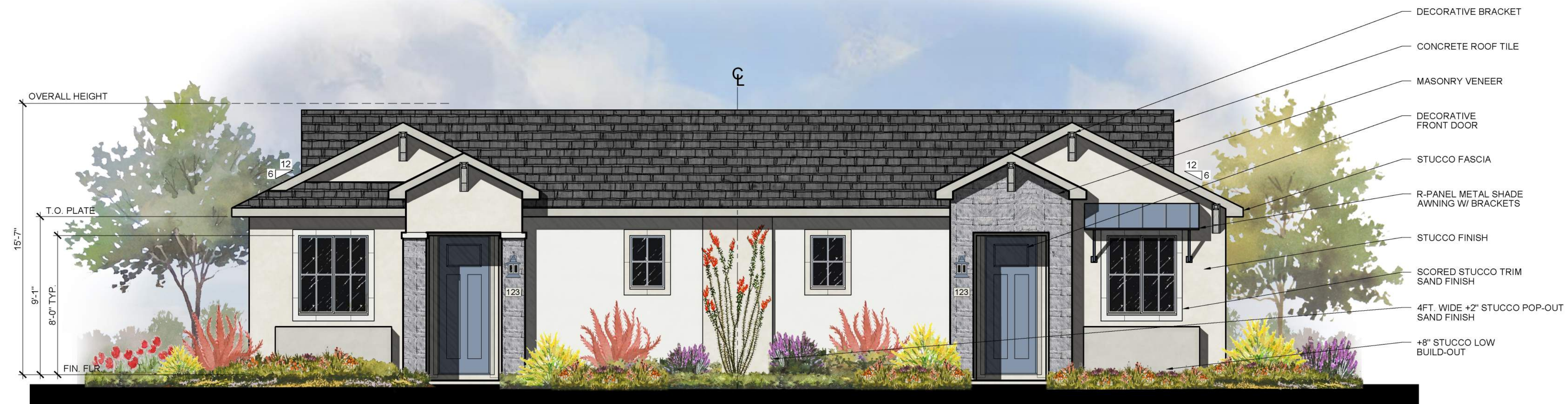
Front Elevation Elevation B 1/4" = 1'-0"
