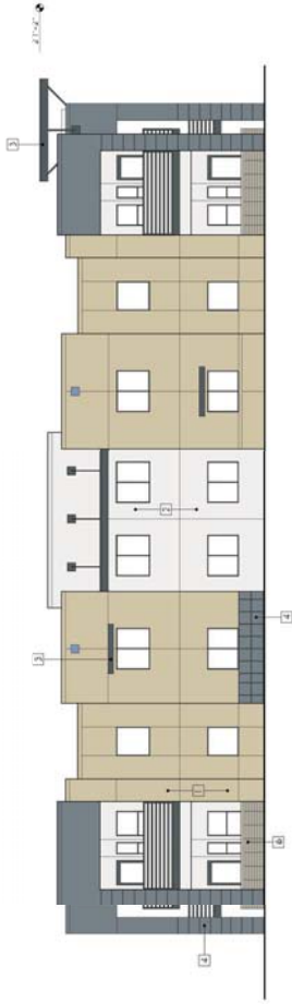
FRONT ELEVATION - BUILDING C1 (3/2-8) (TYPICAL BOTH SIDES)
