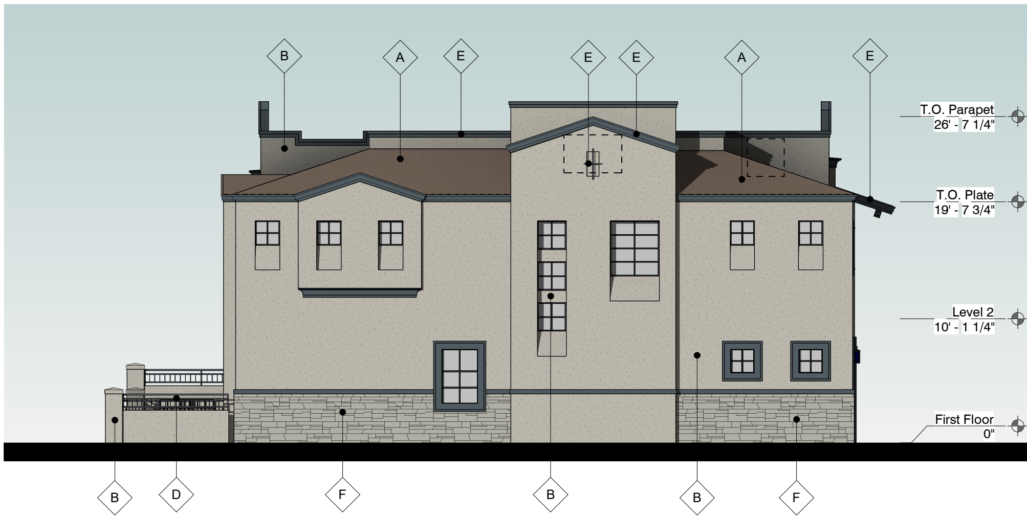
3 Right Side Elevation - 6 Unit Bldg - Scheme 3 1/8" = 1'-0"
