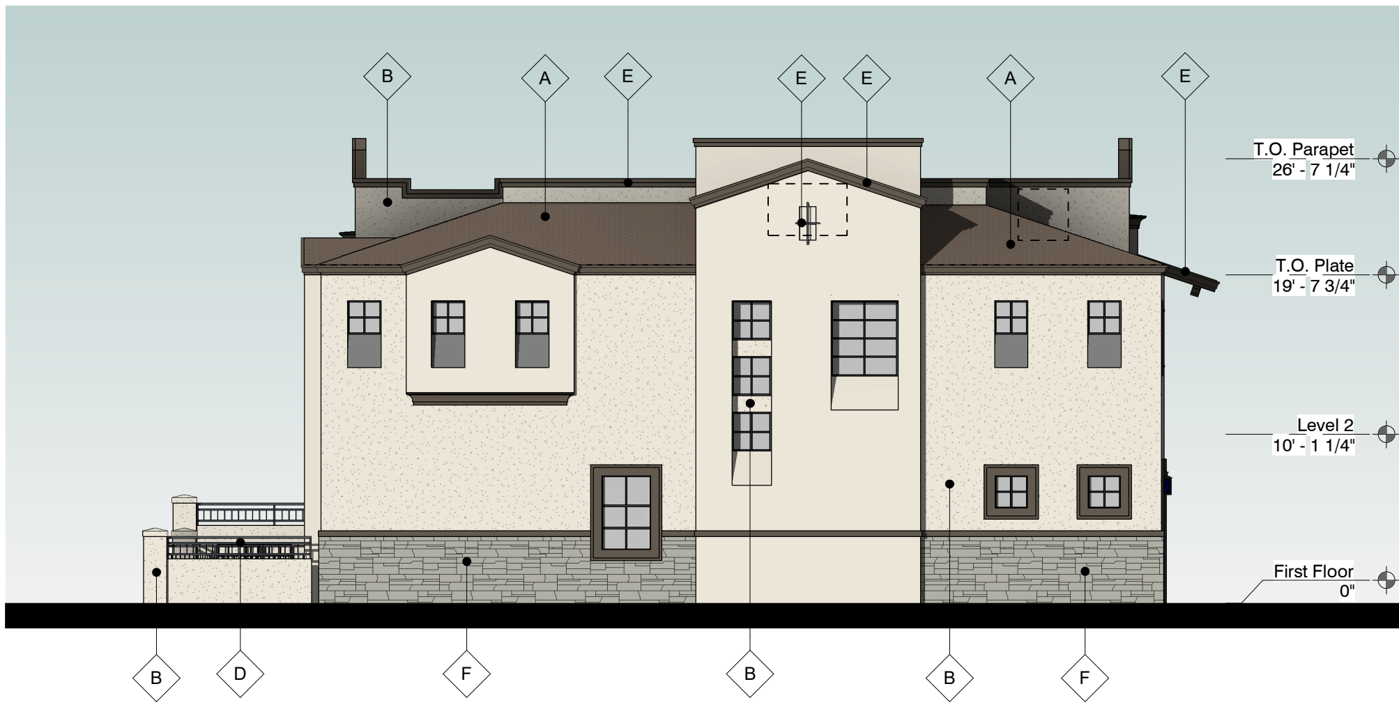
3 Right Side Elevation - 6 Unit Bldg - Scheme 1 1/8" = 1'-0"
