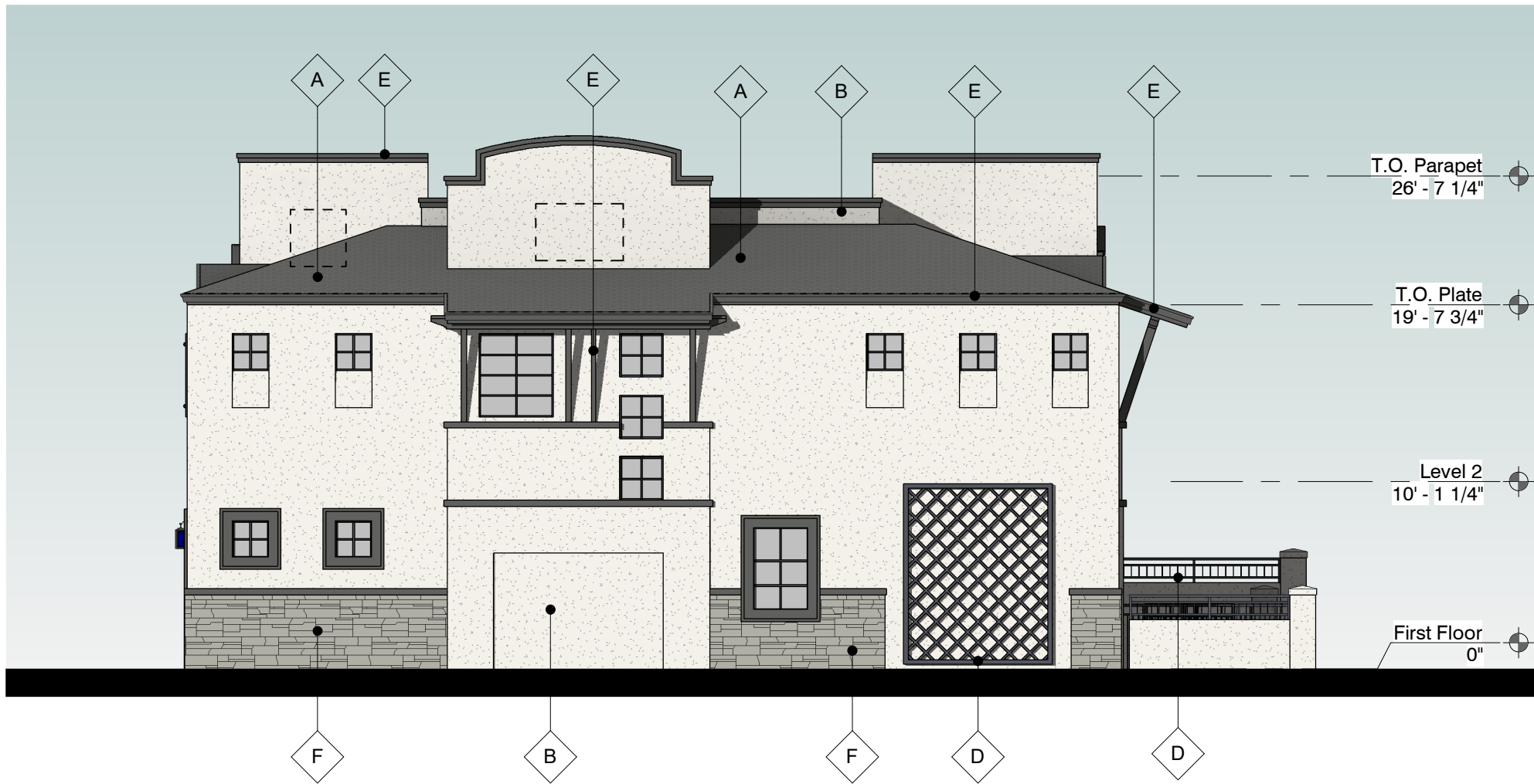
2 Left Side Elevation - 6 Unit Bldg - Scheme 2 1/8" = 1'-0"
