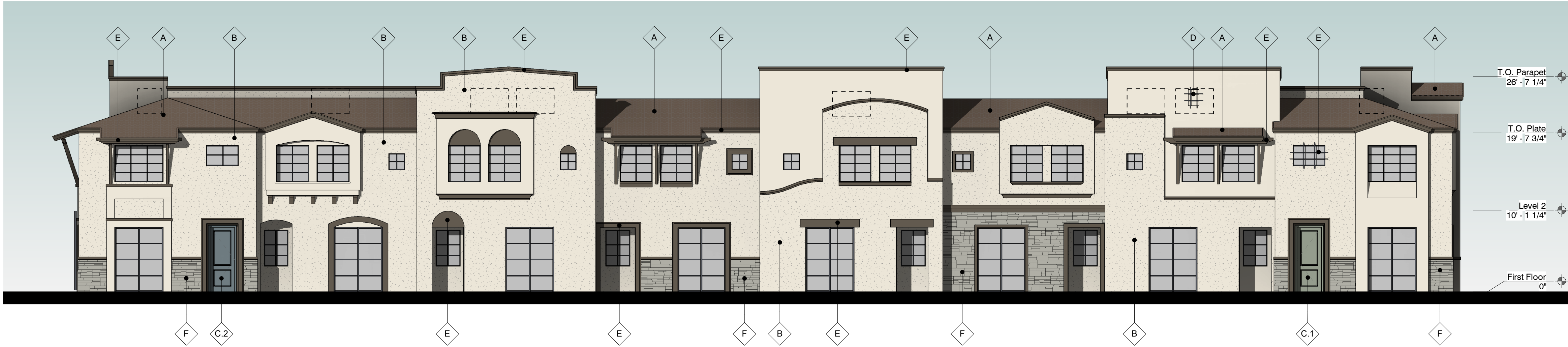
1 Front Elevation - 8 Unit Bldg - Scheme 1 1/8" = 1'-0"
