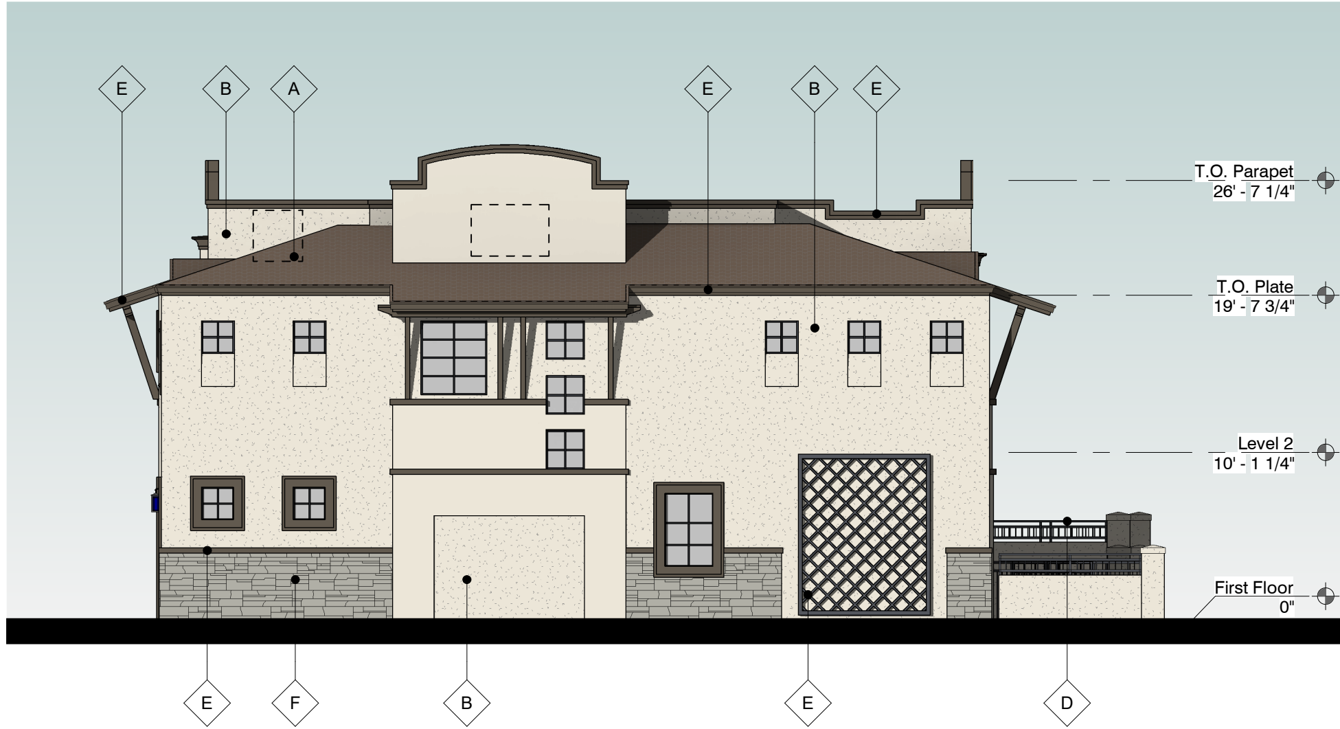
2 Left Side Elevation - 8 Unit Bldg - Scheme 1 1/8" = 1'-0"
