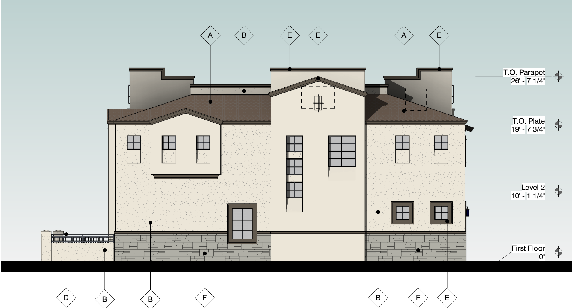
3 Right Side Elevation - 8 Unit Bldg - Scheme 1 1/8" = 1'-0"
